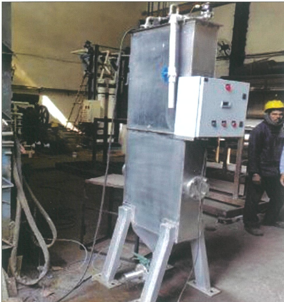
Pilot unit for preliminary pre-trials for demonstration of membrane filtration technology.
